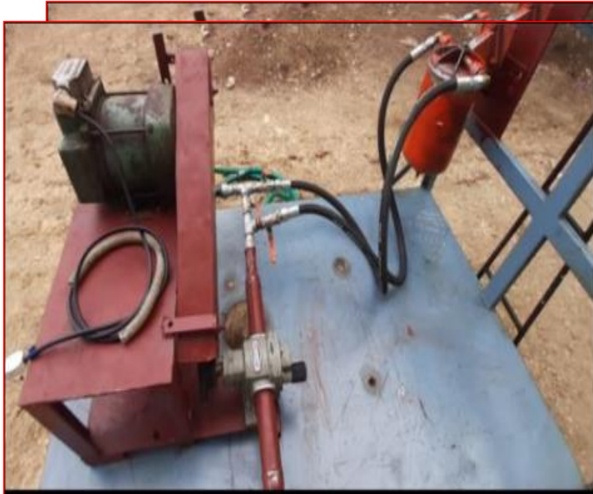
Bio-diesel Filtration unit with Single filter
